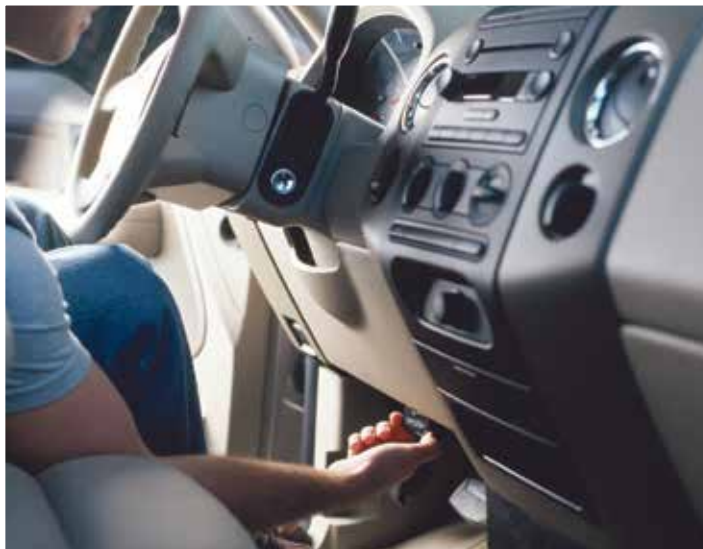
CarChip Connect easily plugs into the vehicle's OBD II port.
